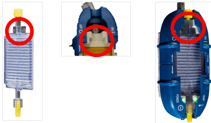
Figure 1. Parylene coated disposable cartridge and warmer have square shape in keying. Circled in red below.
