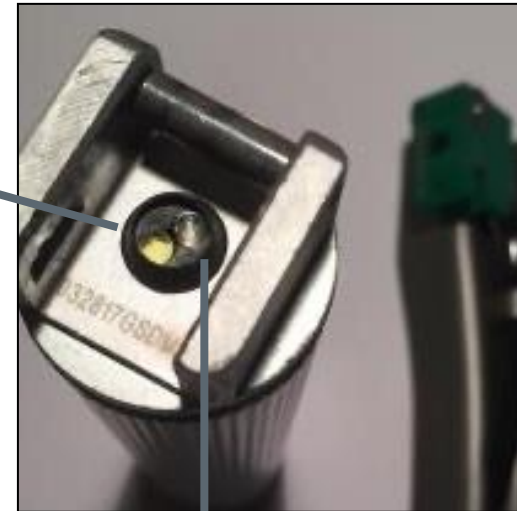
IntuBrite Greenline (Fiberoptic) LED - Two bulbs in handle
